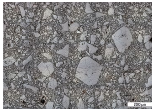
REFRALUSIT® ES matrix Apparent porosity: 18–21%
